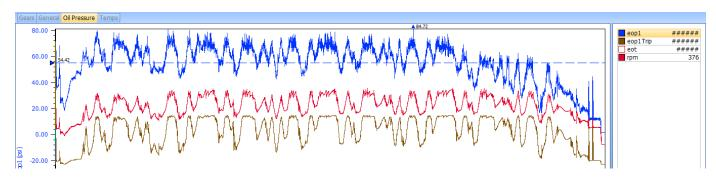
Below is an example of a noisy sensor, the bottom line is what the trace should look like and the top trace contains excessive noise.
