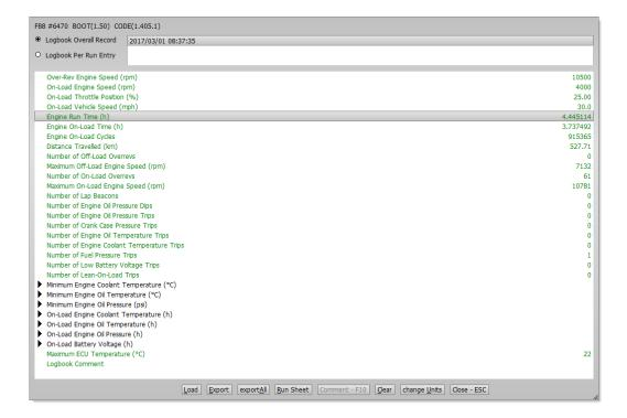
From here LogBook parameters, engine hours and overall recordings can be found. For warranty purposes RPE will reference the total **Engine Run Time** (selected above) Units can be changed using the option at the bottom of the screen
